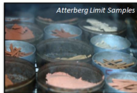
The plastic limit is described as the moisture content of the soil where it transitions between brittle and plastic behavior. This point is determined by rolling the samples in threads 1/8 inch (3 mm) in diameter to the point at which they begin to crack and/or crumble.
