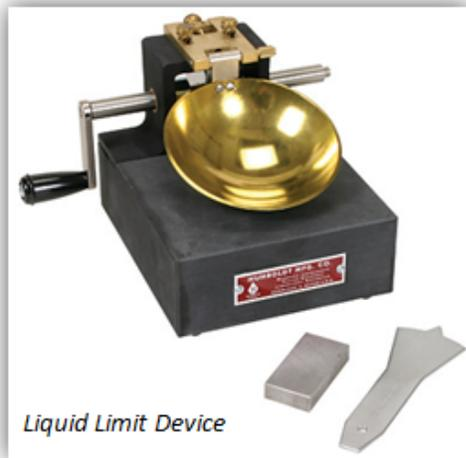
The plasticity index (PI) is the difference between the liquid limit and the plastic limit and provides a description of the moisture states a soil can experience. The PI is an indicator of the potential for expansion or contraction of the soil.
